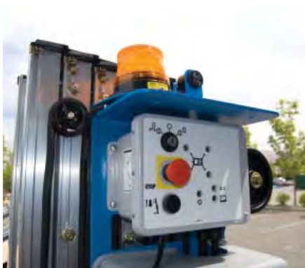
Operational Warning Light
